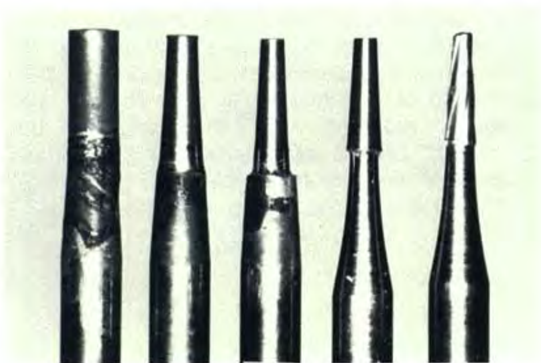
Fig. 3-5 The carbide-tipped blank goes through several machining processes ( left to right ): shortening, head prefinishing, head finishing, neck prefinishing, and head and blade finishing (grinding).*
