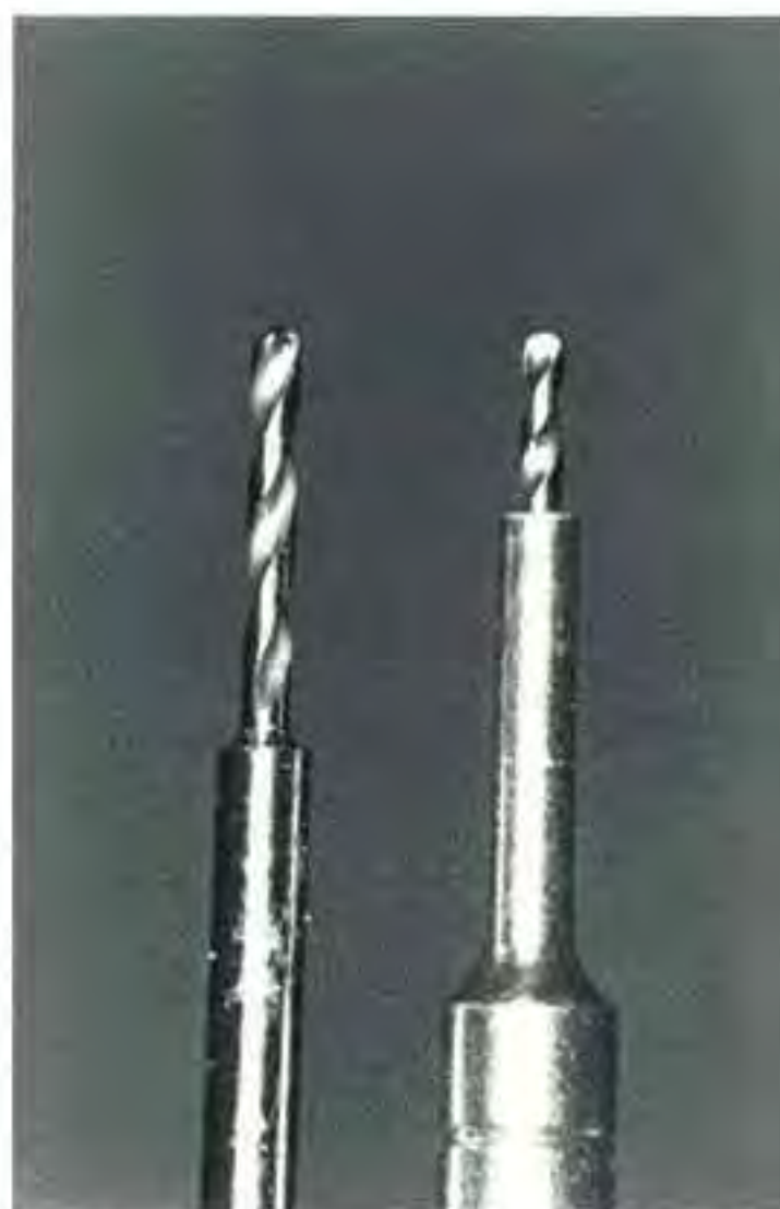
Fig. 3-14 The 0.6-mm-diameter twist drill on the left, used in drilling pinholes for parallel pins, which are an integral part of a cast restoration, has a cutting portion 5.0 mm long.* The 0.5-mm Kodex drill† on the right, used for creating pinholes for Minim threaded pins,† which retain amalgam and composite resin cores, has a collar 2.0 mm from the end to prevent overcutting the depth of the pinhole.
