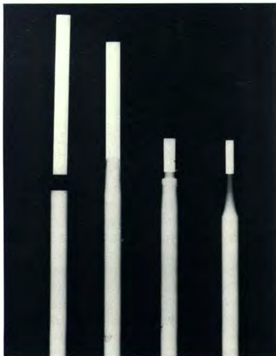
Fig. 3-6 This radiograph shows the carbide blank and steel shaft before ( left ) and after soldering ( second from left ), after initial head finishing ( second from right ), and after blade grinding ( right ). The tungsten carbide segments appear as dense white areas in the radiographs. At this magnification, there are no voids in the attachment areas between the steel shaft and the carbide blank.* (Radiograph courtesy of Ms. Beverly Dye of Oklahoma City.)
