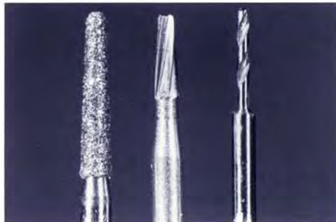
Fig. 3-1 The three types of rotary instruments used in tooth preparation are, left to right: the diamond stone, the tungsten carbide bur, and the twist drill.
