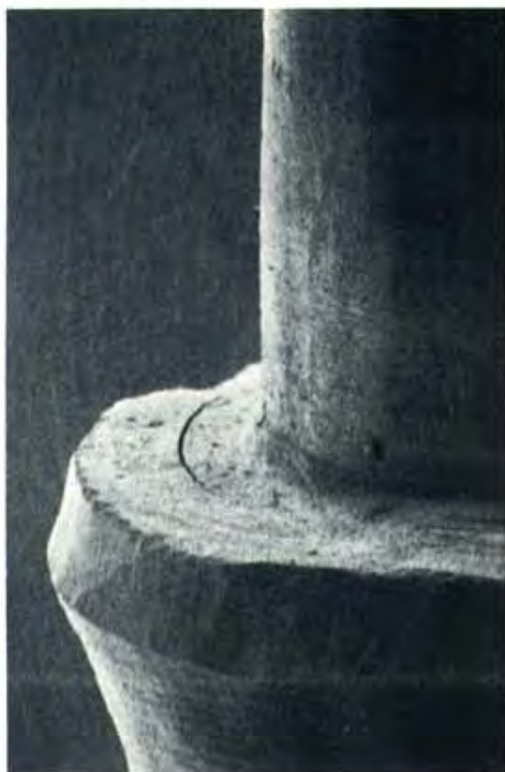
Fig. 3-22 Gingival bevels made with torpedo burs are smoother than those made with diamonds, but the surface is scalloped (35×).
